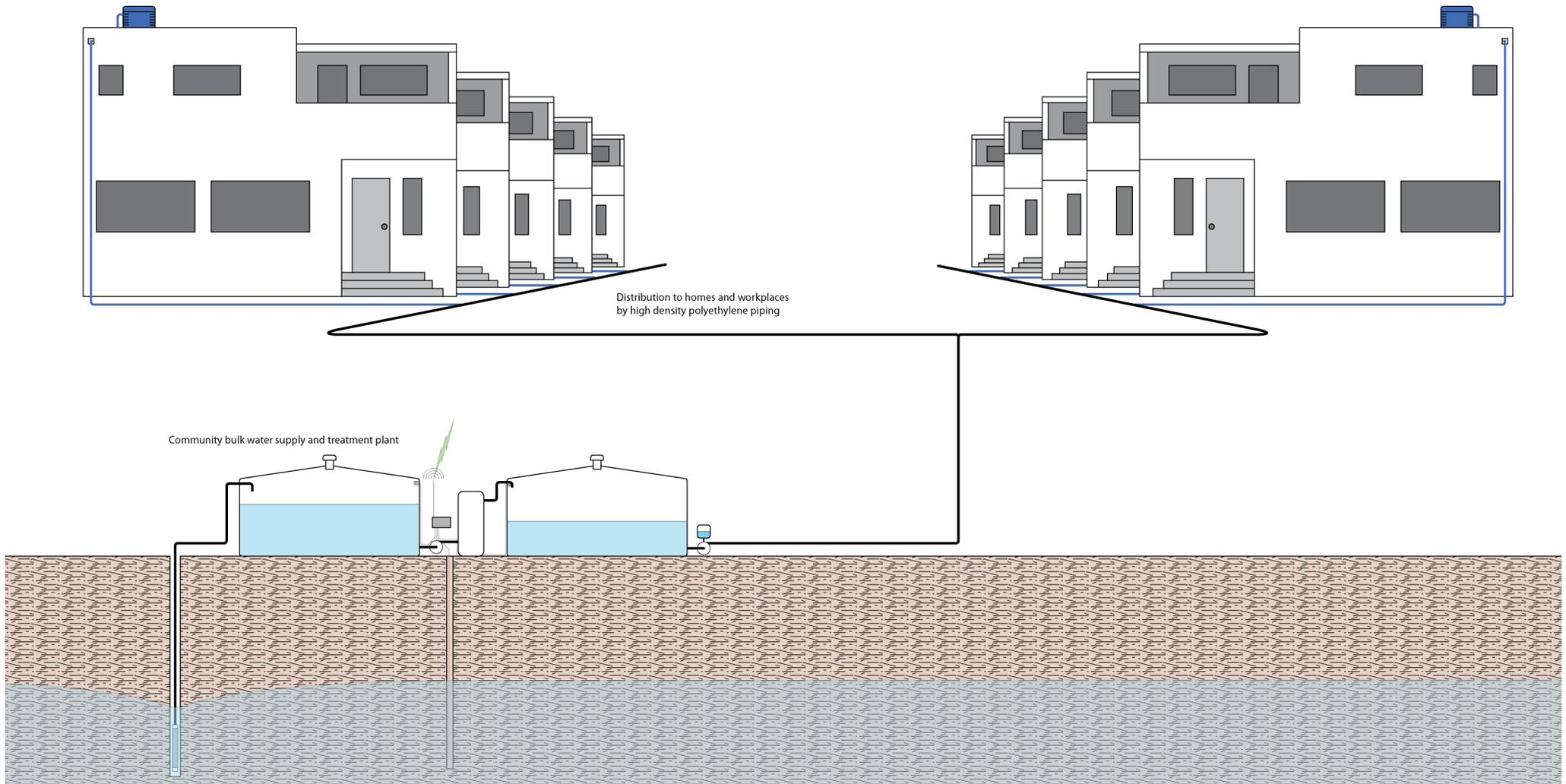
Figure 1: Schematic diagram of drinking water distribution system using ground water for the bulk supply.
