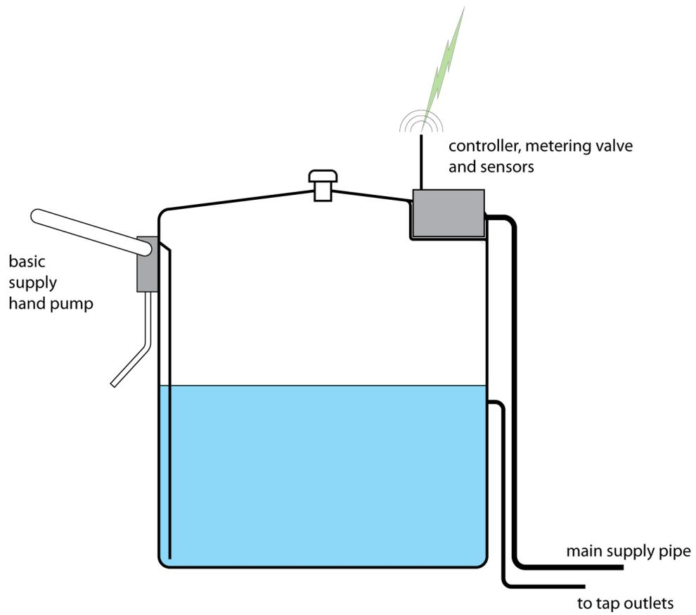
Figure 2: Schematic diagram of building tank
